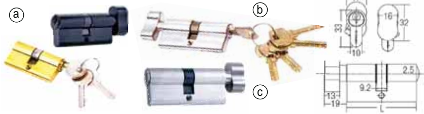
MI-02- a) Double Cylinder b) Thumbturn Cylinder c) Privacy Cylinder Length : 50mm & 60mm & 70mm, 80mm, 100mm Antique Brass / Brushed Satin Nickel / Brass Plated, Matt Black, Satin Black
