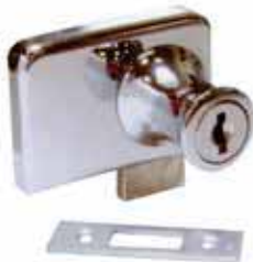
AM-417-5 Cabinet Swinging Glass Door Lock for Double Doors without boring hole on glass and cylinder can be used as handle for glass thickness 5~6mm
