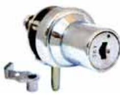
AM 407-1/5 Cabinet Single Swinging Glass Door Lock Without boring hole on glass and cylinder can be used as a knob for glass thickness 5mm-6mm only
