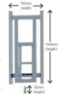
without top and bottom beam Table size : L1300 x W796(mm)
