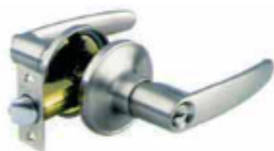
MI-341 CS-XL Tubular Lever Lock Backset : With adjustable latch 80mm - 70mm Functions : Entry, privacy. Colour : Satin Nickel, Polished Brass Rose : 75mm Door Thickness : 35mm - 50mm Backset : 80mm - 70mm
