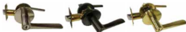
MI-6391L Tubular Lever Lock Backset : With adjustable latch 80mm - 70mm Functions : Entry Colour : Satin Nickel, Matt Black, Satin Brass Rose : 85mm Door Thickness : 35mm - 50mm
