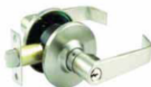
E-841 CS-XL Tubular Lever Lock Material : Zinc Diecast Finish : SN Backset : 80-70mm Door Thickness : 35mm - 50mm Rose : 75mm
