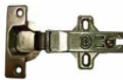
FGV 51A S25050005032 2-Way Slide-on 110° Crank 0, 8, 15mm Cup Diameter: 35mm (Soft closing) (With Detachable Base Plate)
