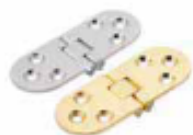
DH-003 Table Flap Hinge Gold Plated, Chrome 70.5mm (w) x 30mm (H) Zinc Alloy / Brass
