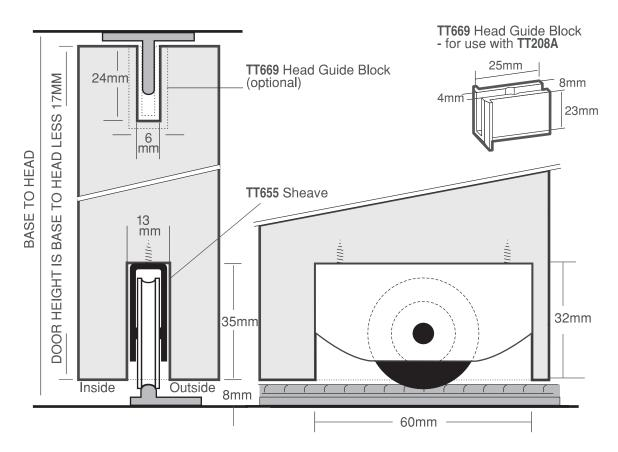
WHERE BI-PASSING DOORS ARE REQUIRED, THE DOOR THICKNESS DETERMINES THE TRACK SPACING.
